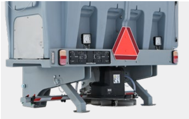
Support legs and dual spray bar, 900-1450 TR
