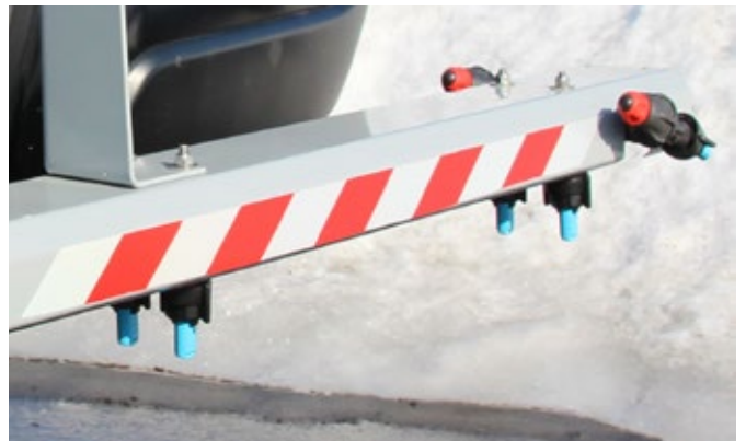
Double spray nozzles for de-icing even at higher speeds
